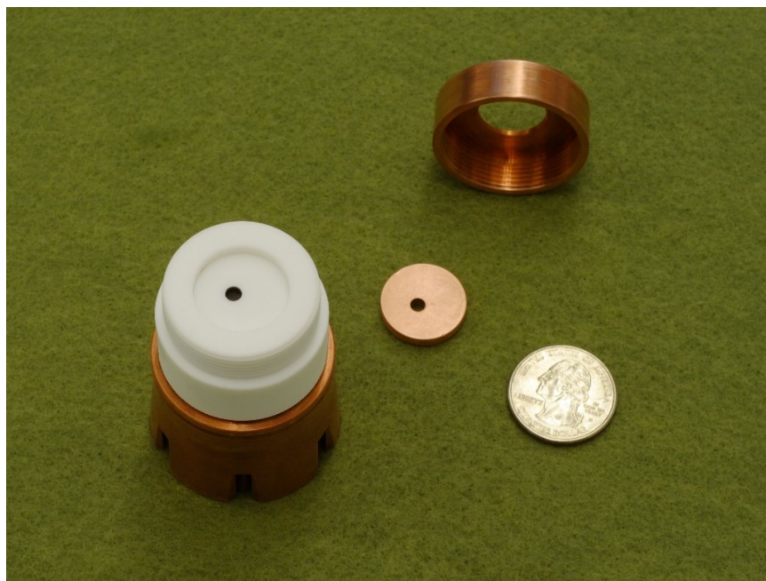
Figure E.2 The target and macor mask are placed onto the cathode base.
