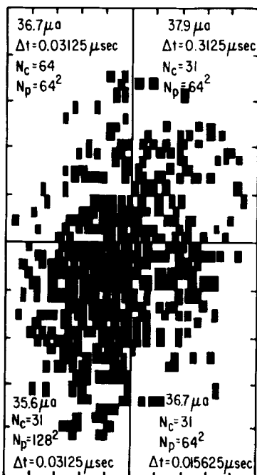
FIG. 20. One quadrant of the UF_6^- charge distribution calculated with the PIC model for a simulation time that is 87.5% of the transit time and for the labelled values of \Delta t , N_c , and N_p . I = 403 \mu\text{A} , R_0 = 2.0 cm, v_1 = 0.316 \times 10^5 cm/sec, \nu_1 = 0.8 MHz, and V_1 = 14.8 kV. The confined flux at 87.5% of the transit time is listed for each calculation. Each tick mark in the horizontal and vertical direction denotes 2.0 cm.
