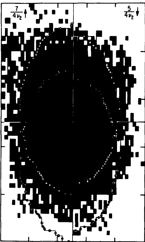
FIG. 16. Calculated symmetric half of the \text{Cs}^+ distribution for times \frac{3}{4}(1/\nu_2) and \frac{5}{4}(1/\nu_2) in (a) and \frac{3}{4}(1/\nu_2) and \frac{5}{4}(1/\nu_2) in (b). The dipole field is applied in the vertical direction, V_2 = 0.1 kV, and there is no quadrupole field. I is 403 \mu\text{A} . The shaded distribution is that calculated with the PIC model. The outlines of both the \text{Cs}^+ (curve with \circ ) and \text{UF}_6^- (curve with \bullet ) distribution calculated in the absence of space-charge coupling are plotted. The arrows indicate the most recent direction in which the applied field attempts to push positive charges. Each tick mark in the horizontal and vertical directions denotes 2.0 cm.
