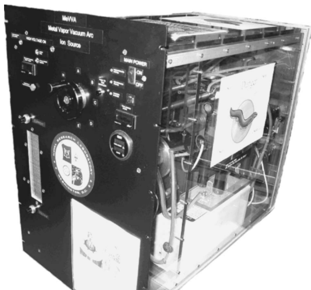
FIG. 2. Photograph of the rack mounted control electronics with the side rf covers removed.
