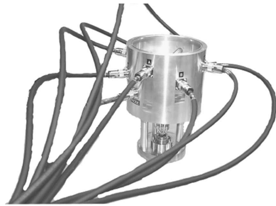
MeVVA head installed on Alignment Fixture
