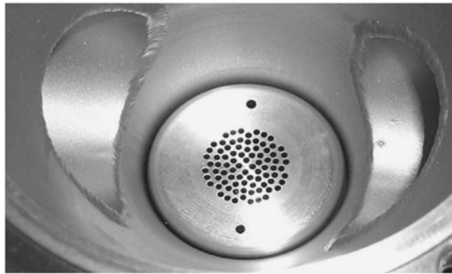
Extractor grid is fixed into bottom of the chamber
